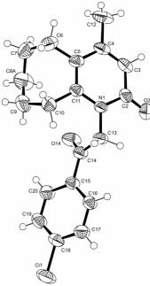
ORTEP-3 (Farrugia, 1997) view of (2), with the atom-numbering scheme. Displacement ellipsoids are drawn at the 50% probability level. Only the major component of disordered atom C8, namely C8A, is shown.
